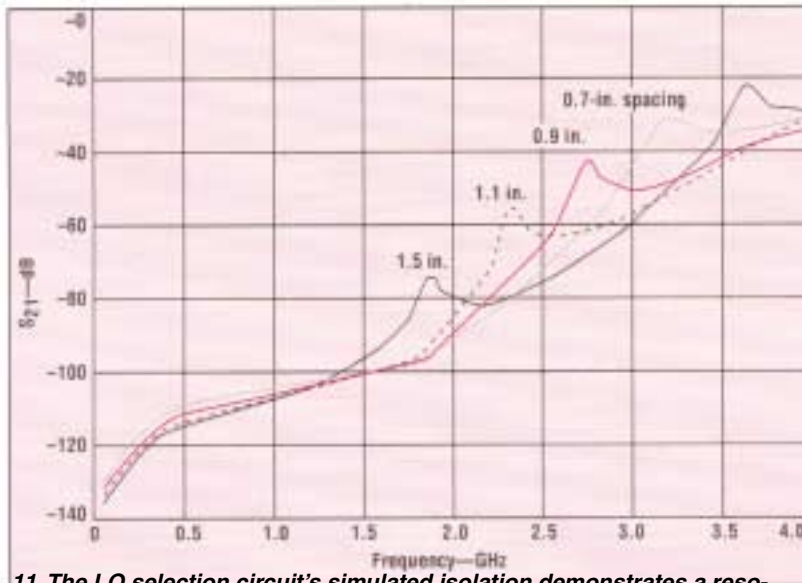
11. The LO selection circuit's simulated isolation demonstrates a resonance that moves down in frequency as the switch spacing increases.
